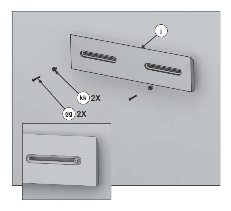
To Mount To Wall, Screw Directly Into Studs When Available.
