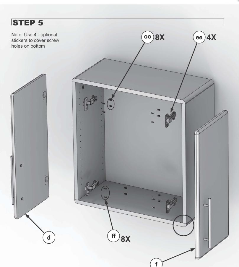
NOTE: Optional Handles should be installed in this step. UltiMATE GARAGE recommends 250mm pulls for GA-09P mounted vertically.
