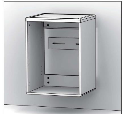
NOTE: For added stability, screw two additional screws into studs through the the top spanner (I) of the cabinet.
