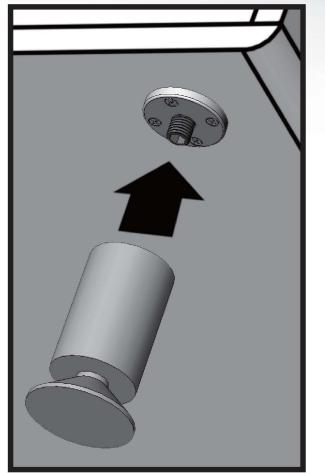
NOTE: Two Front Feet Only or Four Feet can be used with your cabinet. If installing optional feet, do so at this time.
