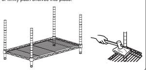
5. Screw the Upper Post (B) into the Lower Post (C) tightly by inserting threaded end of the Upper Post into the open end of the Lower Post.
