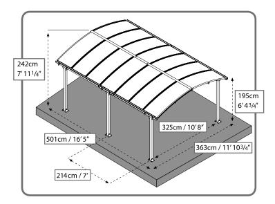
During assembly some screws are fastened fully by wrench while others are fastened just after the whole carport is assembled and leveled (step 21).
