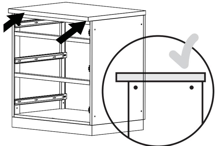
**5** Tighten bolts to secure cabinets.
