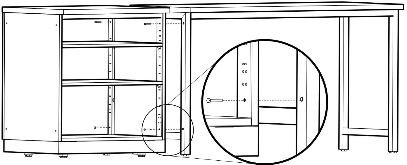
**Note:** Table has rivet nuts in legs to thread into.
