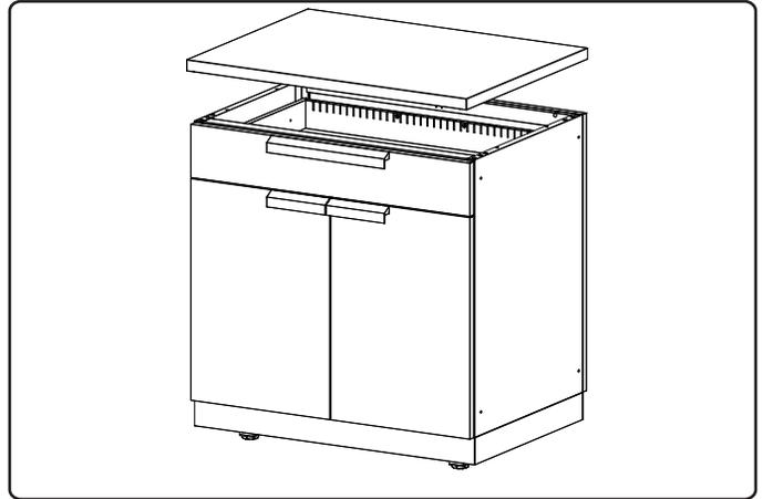
**3** Insert the worktop bolt heads into the keyhole shape slots.
