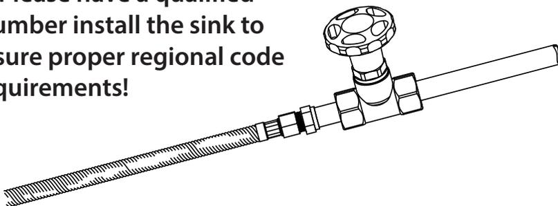
Connect the braided water inlet lines hot and cold to
