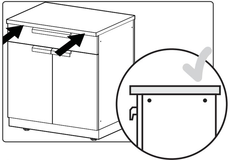
**5** Tighten screws to secure top.
