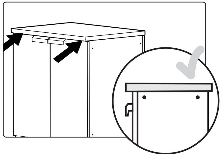
**5** Tighten screws to secure cabinets.
