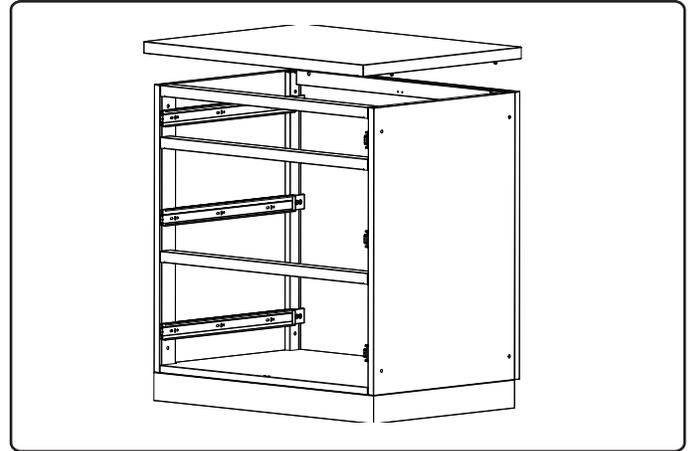
**3** Insert the worktop bolt heads into the keyhole shape slots.
