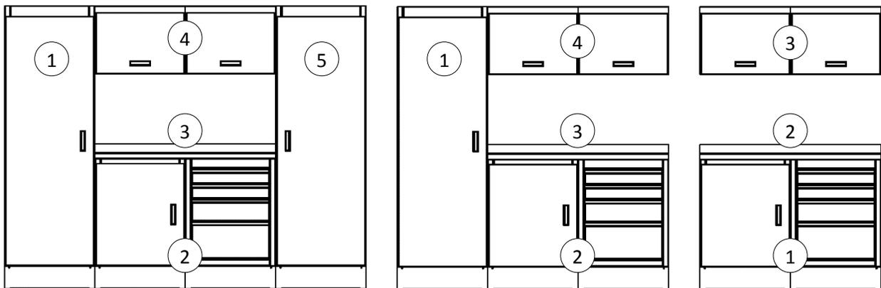
Bolt neighboring cabinets together as you go. Mounting holes are pre-punched, but you’ll need to transfer one front hole from base cabinets, tool boxes or overheads to any adjacent closet.
