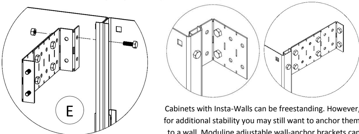
Cabinets with Insta-Walls can be freestanding. However, for additional stability you may still want to anchor them to a wall. Moduline adjustable wall-anchor brackets can accommodate spaces up to 10" from the wall.
