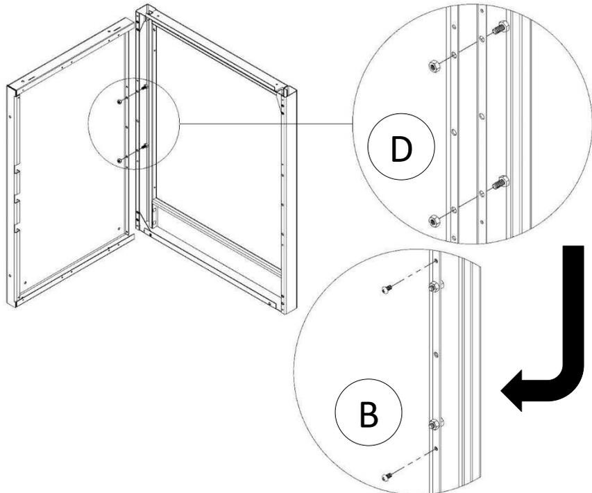
2. Put the counter braces down between the sides and fasten each with (4) 10-24 self-tapping screws **[B]**.
