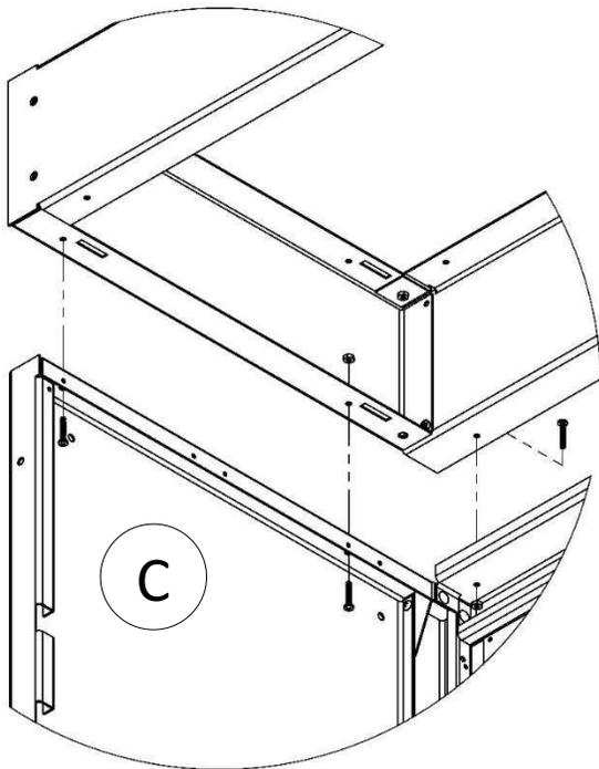
4. Put the toe kick on top of the cabinet and fasten it with (6) 10-32 screws **[C]**. Leave these a little loose for shimming later.
