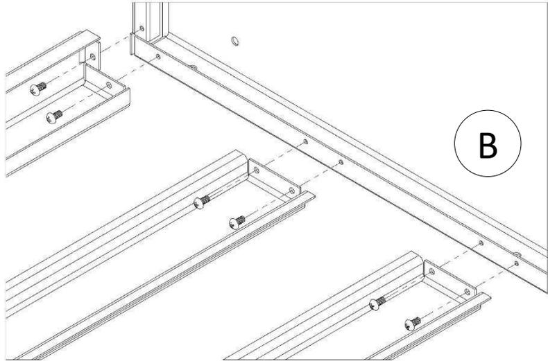
3. Assemble the toe kick with (8) 8-32 flat-head screws **[A]**.
