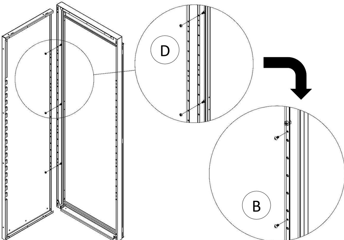
2. Put the closet top down between the sides and fasten with (11) 10-24 self-tapping screws [B].
