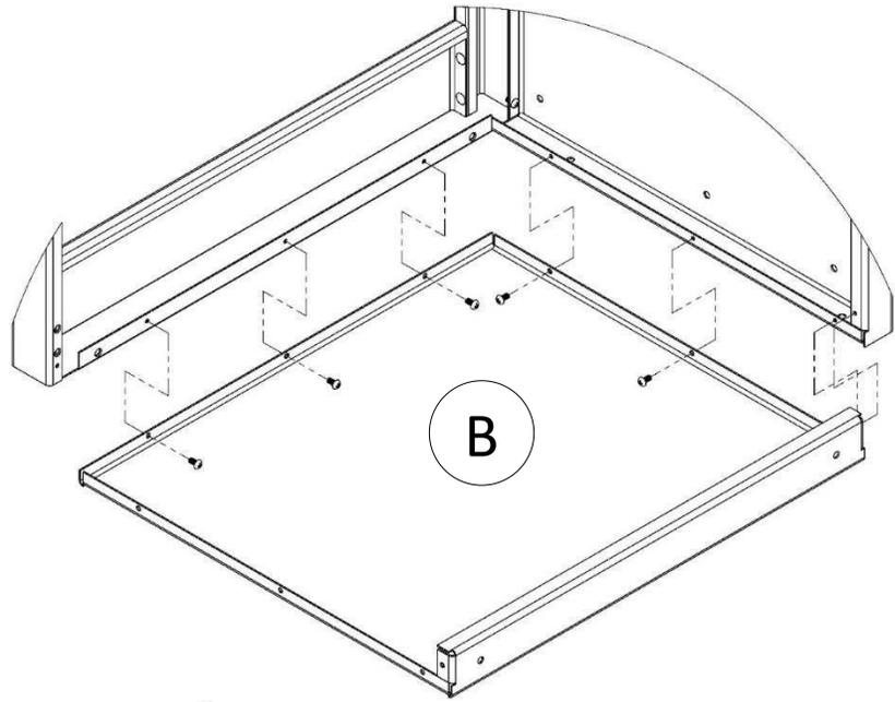
3. Assemble the toe kick with (8) 8-32 flat-head screws [A].
