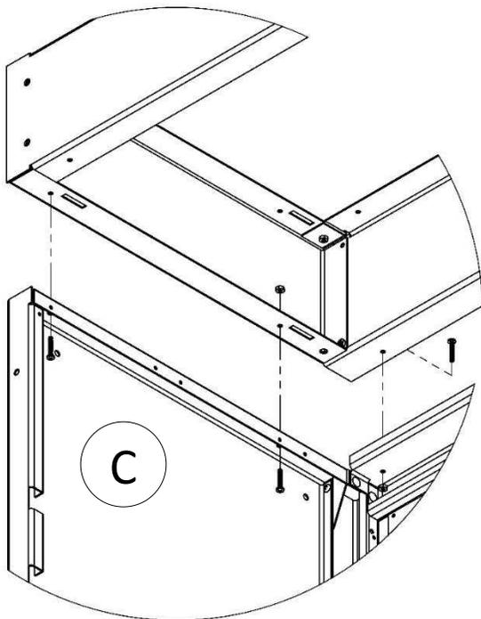
4. Put the toe kick on top of the closet and fasten it with (6) 10-32 x 1" screws [C]. Leave these a little loose for shimming later.
