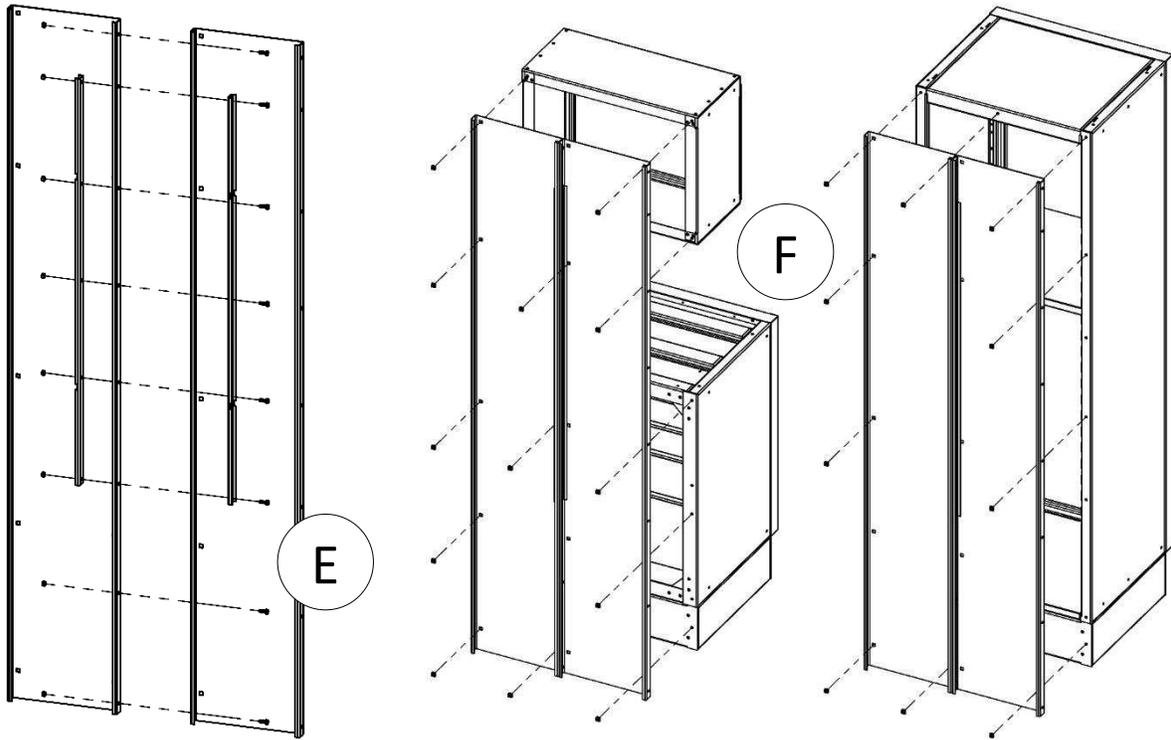
Cage nuts [F] are packed separately. They allow you to mount your cabinets without needing access to the back of the Insta-Walls. Put the cage nuts in the square holes on the back of the Insta-Walls as necessary for each component (see above). Overheads use (5), bases and tool boxes use (8) and closets use (10). **You won't have enough cage nuts to put them in every hole.**
