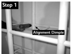
Fasten all Verticals to Horizontals. Make sure all joints are pressed firmly together, tight and against alignment dimples.
