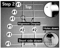
6 Horizontal Crossbars (#1) inserted through 2 Center Verticals (#2) (holes facing down) Tip: When installing second Center Vertical, stand assembly with Horizontal Crossbars placed on floor and push down second Center Vertical to Alignment Dimples.
