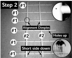
6 Horizontal Crossbars (#1) inserted through 2 Center Verticals (#2) (holes facing up)
