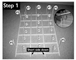
18 Horizontal Sliderails (#7) and 4 Front and Rear Grid Connecting Tubes (#5) inserted in Rear Grid
