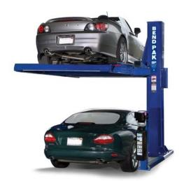
Each stacking system incorporates many distinctive features such as a full-width platform to keep bottom vehicles protected, single hydraulic lifting cylinder combined with heavy-duty leaf chain, automatic safety locks and reliable, ergonomic hydraulic power unit with single-point safety-lock release. These state-of-the-art parking systems are well suited for the typical home garage and utilize a standard 110-volt or optional 220-volt electric-hydraulic power system.
