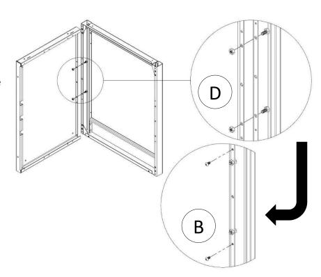
2. Put the counter braces down between the sides and fasten each with (4) 10-24 self-tapping screws [B].
