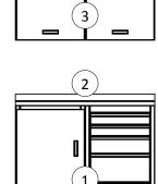
Bolt neighboring cabinets together as you go. Mounting holes are prepunched, but you'll need to transfer one front hole from base cabinets, tool boxes or overheads to any adjacent closet.
