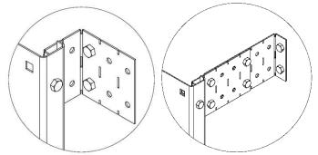
Cabinets with Insta-Walls can be freestanding. However, for additional stability you may still want to anchor them to a wall. Moduline adjustable wall-anchor brackets can accommodate spaces up to 10" from the wall.
