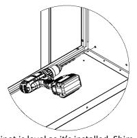
Check that each cabinet is level as it's installed. Shim as necessary using the supplied horseshoe shims. Loosen the toe kick and insert shims between it and the cabinet until level. Bolting the cabinets together can pull them out of square, so you may need to adjust the shims at the end. It's a good idea to shim the cabinets so that they tilt slightly back, especially if you aren't anchoring them to a wall.
